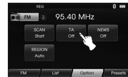
[TA On]: Traffic programs and announcements can be automatically received using TP/TA features.
