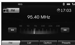
2. Press the "RADIO" repeatedly to select a band. The mode switches as follows. FM → AM → FM...
