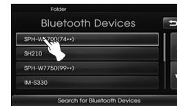
5. Input the passkey (Default: 0000) shown on the screen in your phone when the pop-up screen is displayed on the screen. When it is successfully connected, the Bluetooth main screen appears on the screen.
