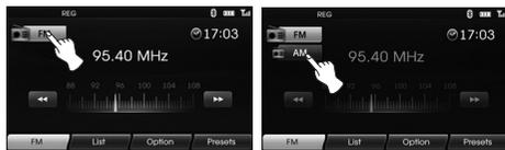
3. **Auto tuning:** Touch **◀/▶** on the screen. Or press **▲/▼** on the control panel.
